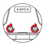
Check whether the inner waterproof ring is in good condition, then install the battery cover and tighten the two screws clockwise.
